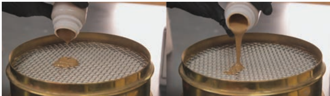
Fig. 6—Comparison of Baker Hughes' NSURE drilling fluid, right, with conventional fluid, left, at 9°F.
