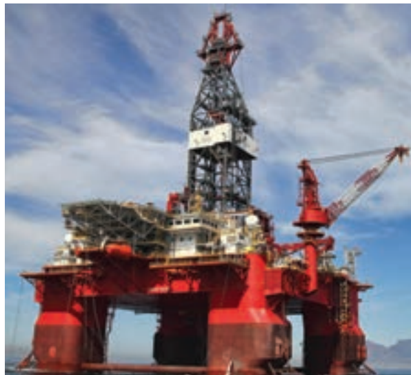
The Ocean Valor, owned by Brasdril, is one of two rigs equipped by Petrobras for managed-pressure drilling in deep water. It was used to finish a well in the Lula field that could not be completed using conventional methods. Courtesy of Petrobras.
