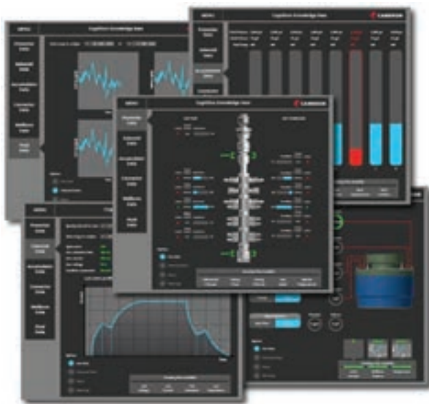
Cameron introduced its BOP monitoring system, Cognition, at this year's Offshore Technology Conference in Houston. The system monitors the condition of every moving part in a BOP by interpreting the electrical signatures produced when each component is actuated. Image courtesy of Cameron.
