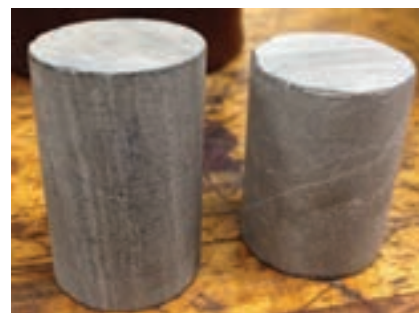
Fig. 1—Preserved sidewall Cores 1 and 2 after the first experiment.
