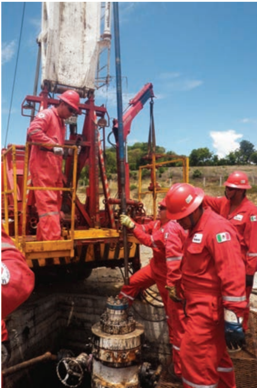
Fig. 2—Weatherford employees prepare to run the Flexisert I-PCP anchor into a well in Poza Rica, Veracruz, Mexico.
