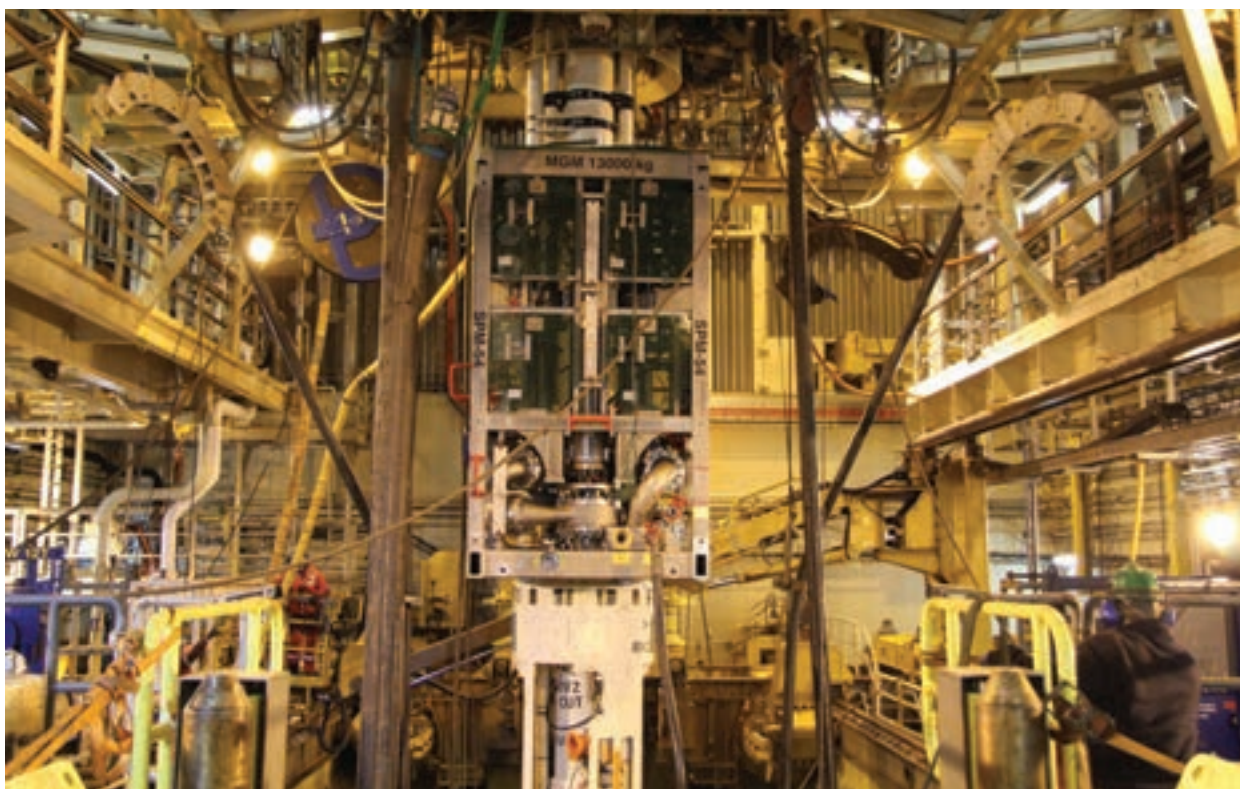
The EC-Drill pump is connected to the riser in the moonpool of the COSL Innovator which was used to drill wells using the dual-gradient system in the Troll field off Norway. In the bottom of the metal frame are the pumps and in the lower middle is a motor. Courtesy of Enhanced Drilling.
