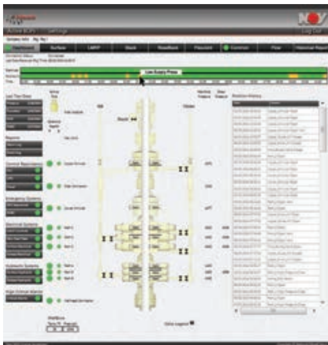
NOV's BOP monitoring system, eHawk, uses a color-coded dashboard system to indicate the level of risk associated with each component. The company is running a pilot program with the system on two Ensco drillships operated by BP. Image courtesy of NOV.
