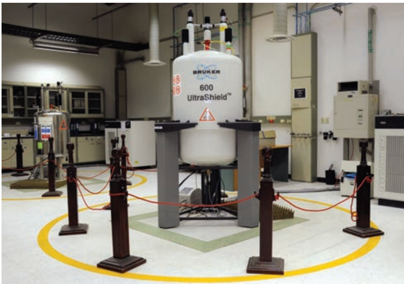
A 600 MHz Bruker UltraShield NMR (nuclear magnetic resonance) spectrometer for liquids analysis at Qatar Science and Technology Park.
